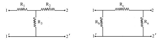
Show that these networks will be equivalent in the sense that the resistances between the corresponding pair of terminals will be identical provided
